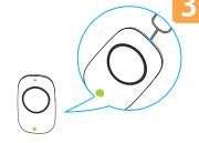
According to APP prompt, press the button for 2 seconds, green LED flash quickly, APP Interface prompted, networking success. (Press networking hole for 5 seconds if any changes for internet, green LED flash slowly for 3 seconds, exit network successfully
